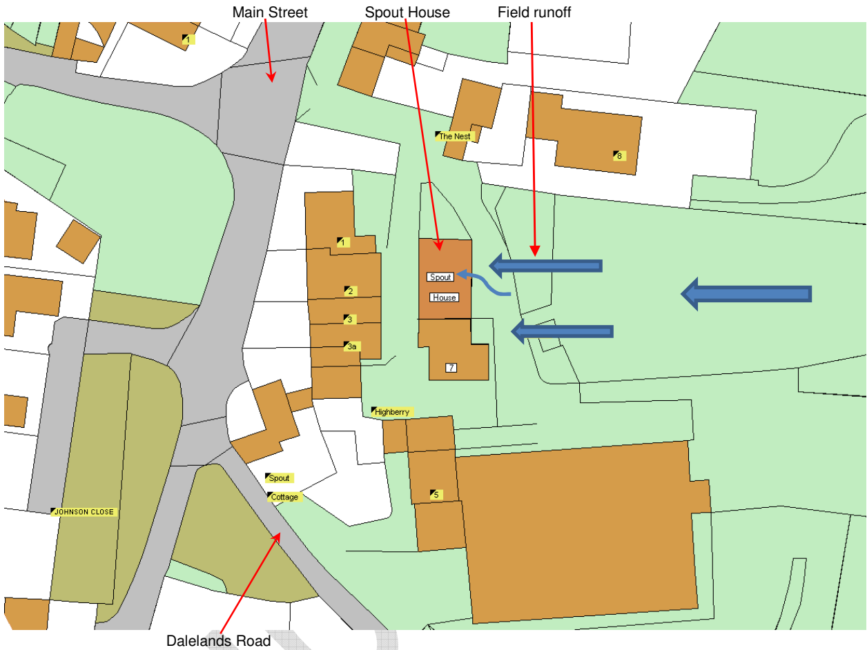
Figure 6: Spout House Flood Routes
