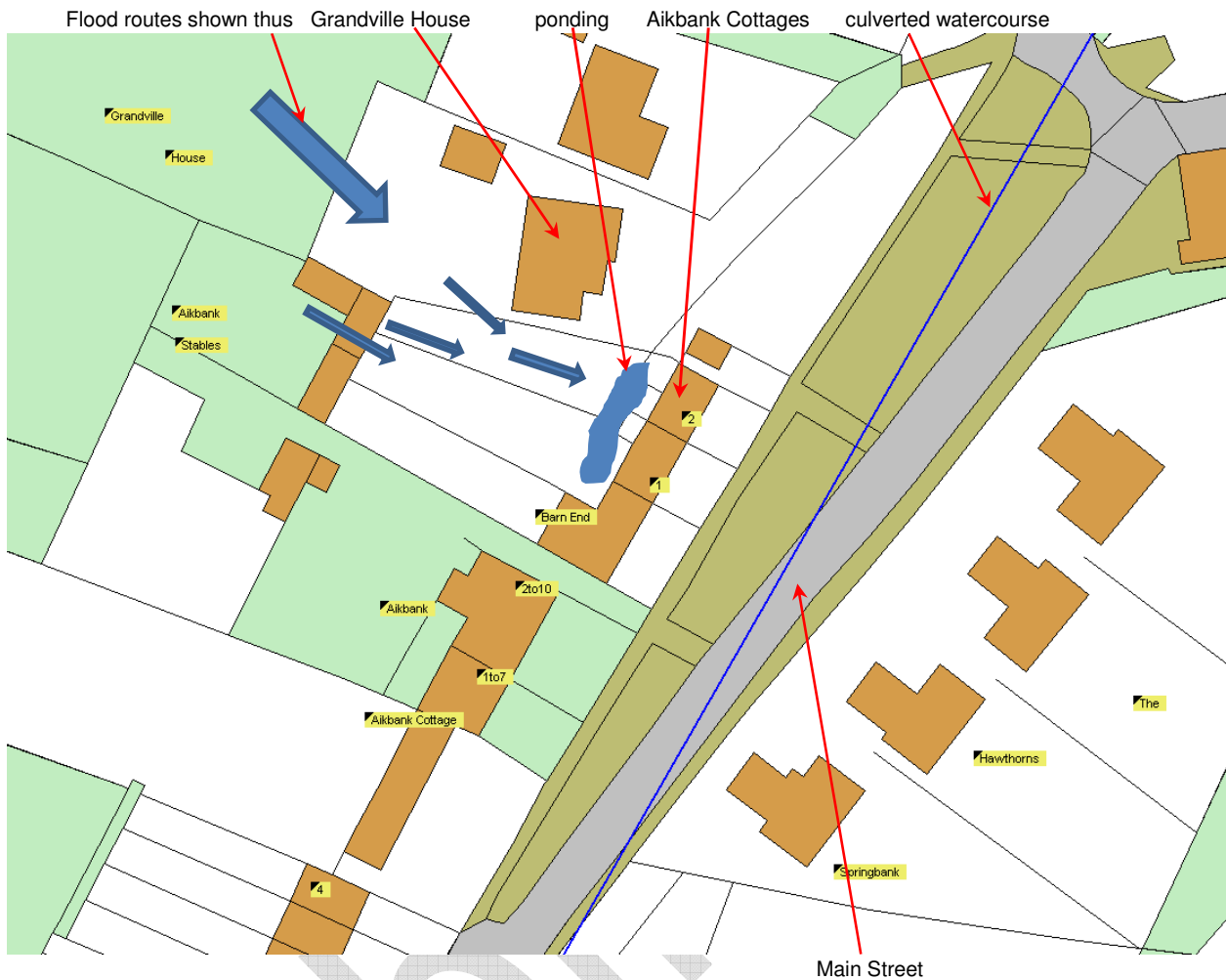
Figure 7: Previous Aikbank Cottages' Flood Routes.
