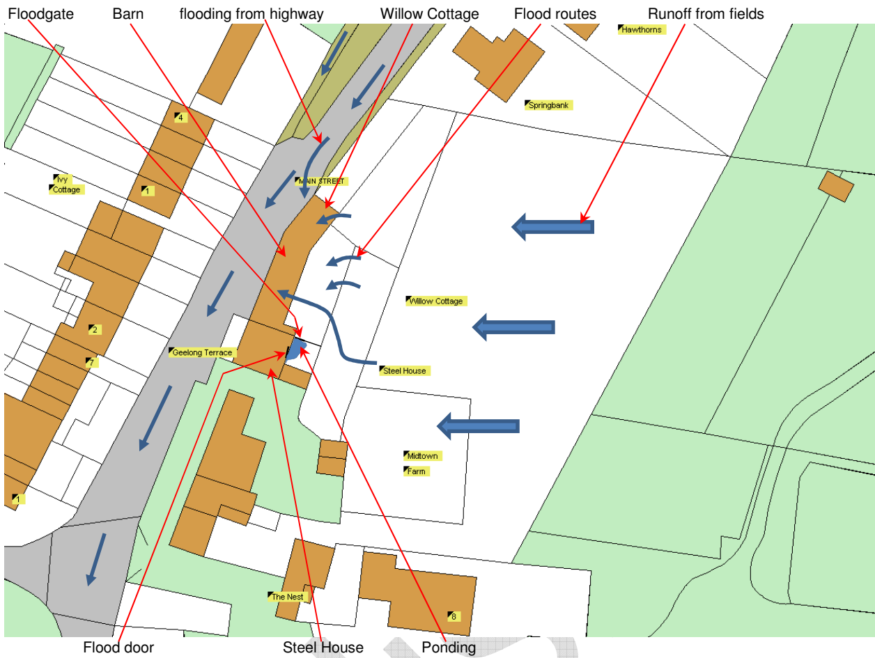
Figure 5: Steel House Flood Routes.
