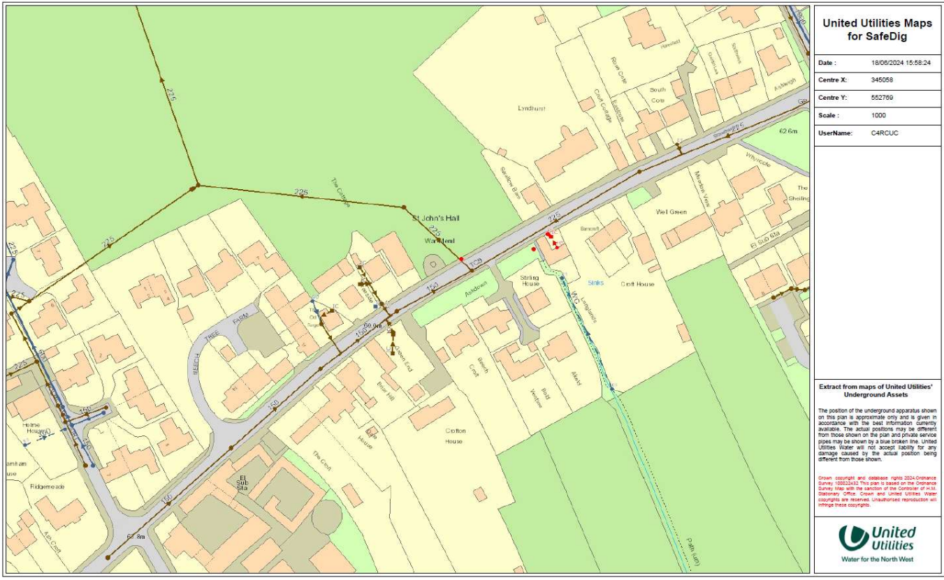
Figure 10: United Utilities map showing location of sewers
